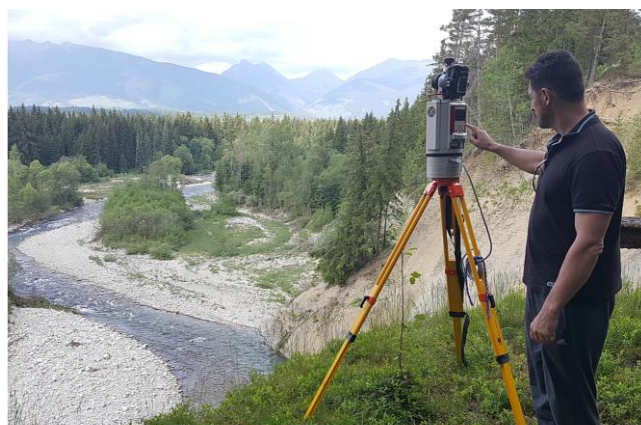
Laser scanning bank erosion in the High Tatras with the RIEGL VZ-1000.
